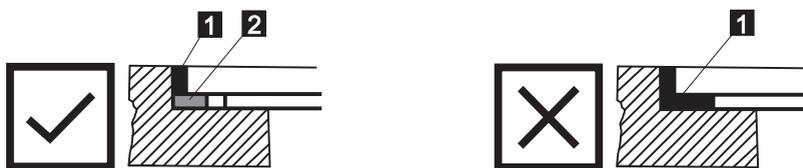
1. Silicone sealant, 2. Sealing tape
