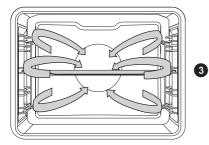
Round heater and the fan will operate. The fan installed on the back wall of the oven cavity makes sure the hot air constantly circulates around the meat, vegetables, or pastry.
