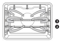
In the Auto Roast mode, the upper heater will operate in combination with the grill heater and the round heater. It is used for roasting all types of meat.
