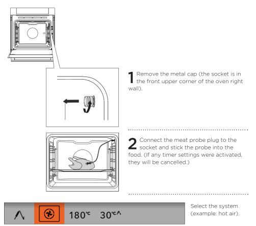
Preset temperature and probe temperature will be displayed. Set the cooking system and temperature, and the final temperature of the dish. Touch the START key.
