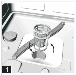
Step 1: contrarotate the Coarse filter , then lift it up;
