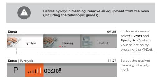
Depending on the model: There are three available cleaning intensity levels. The more stubborn the dirt, the higher level should be selected.
