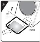
Incline the machine to an angle of 40° and let the side with right-angle notch face towards front of the washing machine, as shown in the figure. Insert the side with oblique-angle notch between two foot screws at back of the washing machine completely in place. Then, install the bottom plate and ensure that it contacts with bottom of the washing machine closely.
