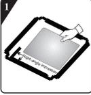
Before installing the noise-reduction bottom plate, align and paste the acoustic absorption wool with and along the right-angle impression on bottom plate (this procedure is unnecessary for some of the models without acoustic absorption wool).
