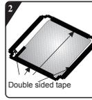
Remove surface paper on double sided tape at four sides of the bottom plate.
