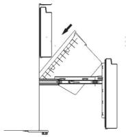
Put the tray on the drawer and push it award and ensure the tray's rollers on the freezer liner (D)'s fillets.
