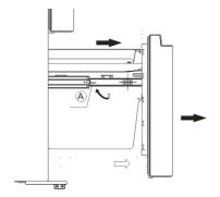
3. Take out the tray (B) by lifting it up in the direction of the arrow.
