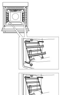
${\sf A}$  Hold the guides by the bottom side and pull them towards the center of the oven cavity.
