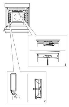
**1** Unscrew and remove the cover (in anti-clockwise direction). Remove the halogen bulb.
