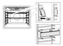
Click-on pull-out guides can be attached in any space between two wire guide levels. Place the guides symmetrically onto the wire guides on the left and right side of the oven cavity. First, hook the upper clip of the guide onto the wire of the wire guide. Then, press the lower clip into the right position until you hear a click.
