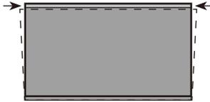
If the top of the image is narrower than the screen, then use the wrench to rotate the left- and right-back feet of the Laser TV clockwise, until the left and right borders of the image are parallel with the screen borders.
