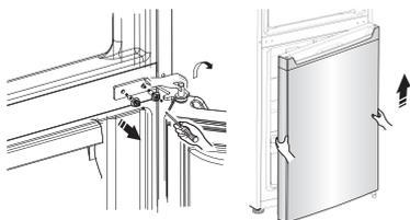
8. Place the lower door on a smooth surface with its panel upwards. Loose screw ② and part ①, then install them to the left side and tighten securely.
