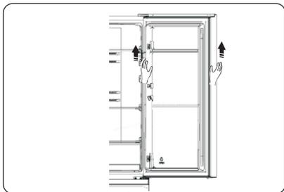
6. Place the upper door on a smooth surface with its panel upwards. Loose screw ② and part ①, then install them to the left side and tighten securely.
