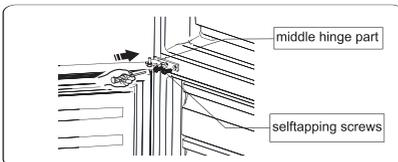
14. Transfer the upper door to the appropriate position. Secure the door's level, make the middle hinge axis into the lower hole of the upper door.
