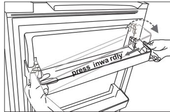
Firstly tilt the left side of the door shelf, and make sure the notch has been fastened to the door. Then press the right side inwardly, push it down to the right place.
