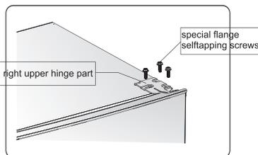
4. Remove the upper hinge axis, transfer it to reversed side and tighten securely, then put it in a safe place.
