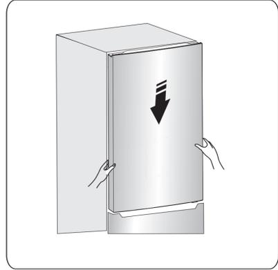
15. Transfer the upper hinge part and make the upper hinge axis into the upper hole of the upper door, and adjust the position of the upper door (please support the upper door with your hand when doing it), fixing the upper hinge part with the special flange self-tapping screws.
