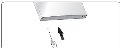
7. Unscrew the two special flange self-tapping screws which are used for fixing the middle hinge part, then remove the middle hinge part that holds the lower door in place.
