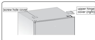
3. Unscrew the special flange self-tapping screws which are used for fixing the right upper hinge part by a 8mm socket wrench or a spanner (please support the upper door with your hand when doing it).
